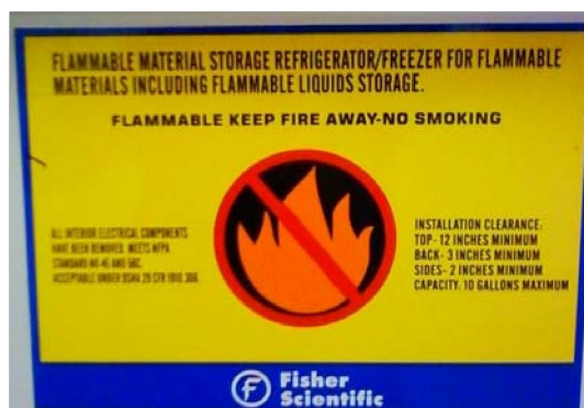
Figure 2 – Flammable Refrigerator Sign
