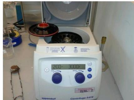
2. Place samples in a slot making sure the rotor is balanced while rotating (if 2 samples, place 1 across from the other)
