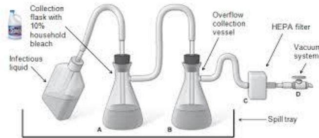
**Figure 5 – Example of Aspiration Flask Set-up**
