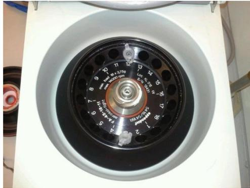
3. Close the rotor and lock it in place by turning it clockwise until a clicking noise is heard.
